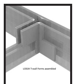
The LOGIX T-walls easily assemble with snap-in ties. The ties are the same ties used for LOGIX KD forms. In addition, the T-wall panels are 2.75 inches thick, which makes the LOGIX T-walls fit seamless with LOGIX KD and PRO forms.
