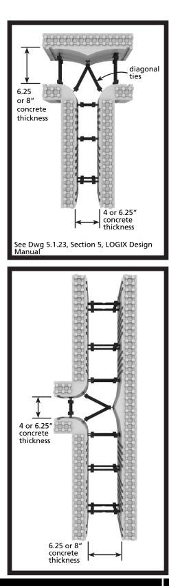
LOGIX T-wall forms were designed with strength and efficiency in mind. The end result are T-wall Forms that provide builders a fast, efficient way to construct t-junctions with minimal waste, little effort, and the comfort of knowing builders are working with a safe, strong, building product.
