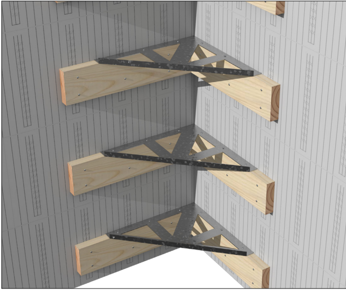
STEP 3: 2x4 strapping and Buck Braces should be attached at every course of ICF installed. Make sure to add the required reinforcement as each course is installed.
