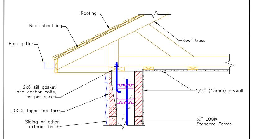
See Section 6 — Engineering in the LOGIX Product Manual for reinforcement details.
