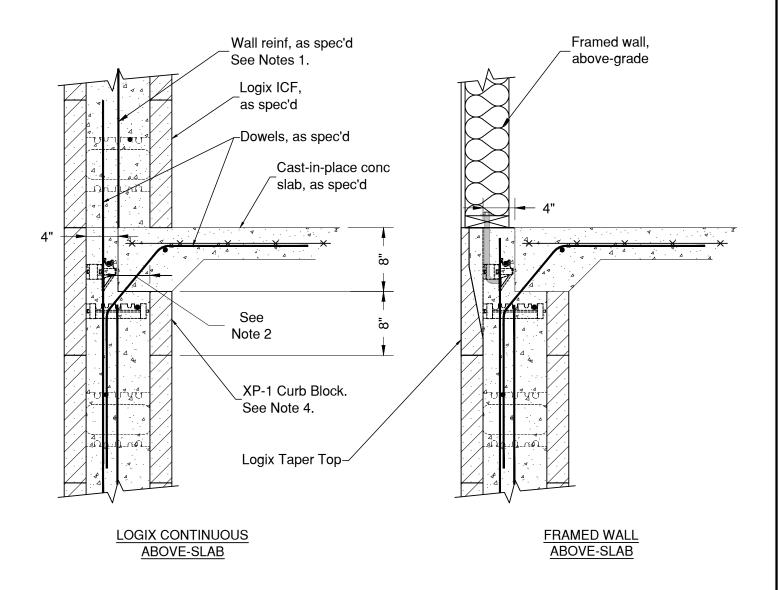
For wall reinforcement refer to the Logix Design Manual, Secdtion 6 Engineering.
