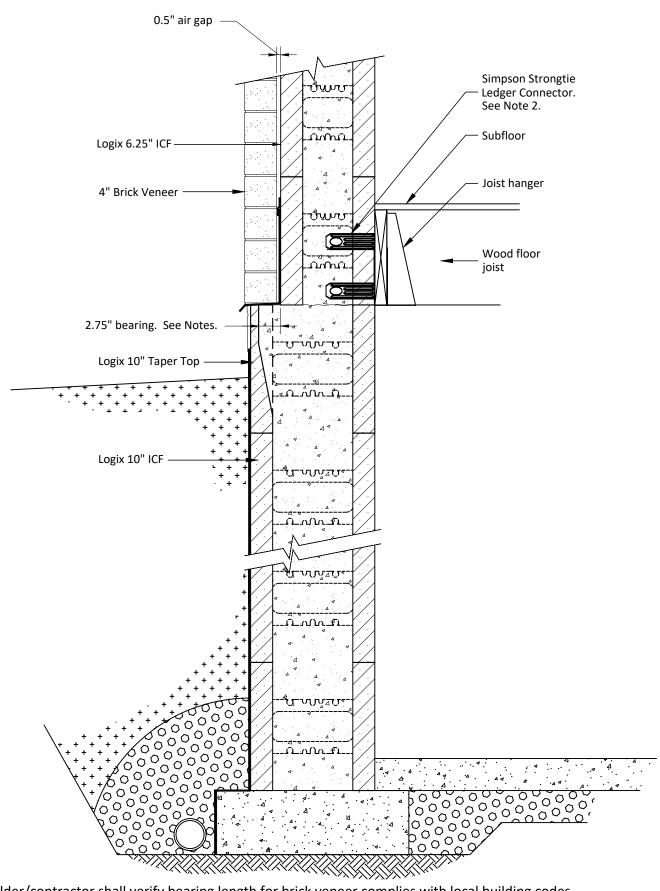
1. Builder/contractor shall verify bearing length for brick veneer complies with local building codes.
