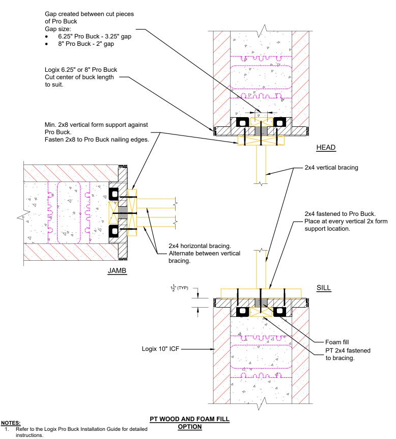
At sill location provide min. 4" diameter access ports to allow for adequate concrete placement and consolidation.
