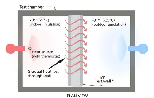
Amazingly, for 2 entire days, the thermostat did not detect a temperature drop and the heat never turned on! **THEN**, for days 3 and 4, the R-24 ICF wall actually operated at an amazing R-45\*\* to R-82\*\* **AND** for the 10 remaining days of the test, the ICF wall operated from R-45\*\* and gradually tapered down to its actual R-24 R-value on day 14 where it remained thereafter.
