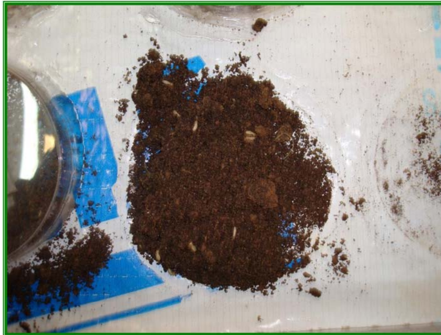
Termites over Colphene ICF
