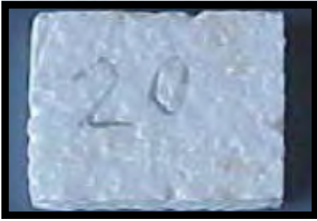
Termite attack on EPS treated with Imidacloprid
