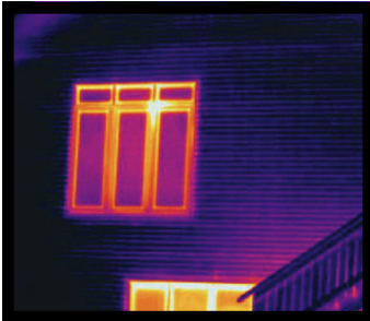
Thermal image of exterior LOGIX wall showing no heat escape through the wall. Continuous thick insulation with a solid concrete core wall prevents thermal bridging and heat escape through LOGIX walls.
